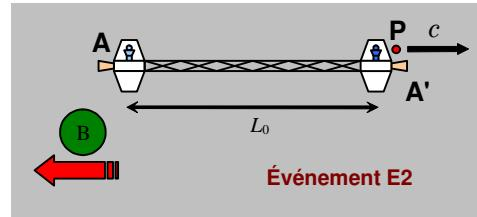
Durée :  $T_A = \Delta t_A = t_{A(2)} - t_{A(1)} \Rightarrow T_A = \frac{L_0}{c}$     (Remplacer  $t_{A(1)} = 0$  et  $t_{A(2)} = \frac{L_0}{c}$ )
