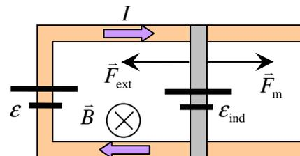
$$\begin{aligned} \sum \Delta V = 0 &\Rightarrow \epsilon_{\text{pile}} - \epsilon_{\text{ind}} - RI = 0 \\ &\Rightarrow (12) - \epsilon_{\text{ind}} - (3)(1) = 0 \\ &\Rightarrow \boxed{\epsilon_{\text{ind}} = 9 \text{ V}} \end{aligned}$$
