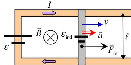
$$v(t) = v_{\text{lim}} \left[ 1 + \left( \frac{v_0}{v_{\text{lim}}} - 1 \right) e^{-\frac{\ell^2 B^2}{mR} t} \right]$$
