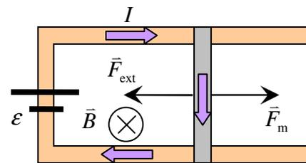
$$\begin{aligned} \sum F_x = 0 &\Rightarrow F_m + F_{\text{ext}} = 0 \\ &\Rightarrow F_m + (-0,2) = 0 \\ &\Rightarrow \boxed{F_m = 0,2 \text{ N}} \end{aligned}$$
