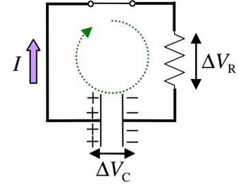
$$\begin{aligned}\Delta V_C + \Delta V_R = 0 &\Rightarrow \left(\frac{q}{C}\right) + \Delta V_R = 0 && (\Delta V_C = +q/C) \\ &\Rightarrow \frac{q}{C} + (-RI) = 0 && (\Delta V_R = -RI) \\ &\Rightarrow \boxed{I = \frac{q}{RC}} && (\text{Isoler } I)\end{aligned}$$
